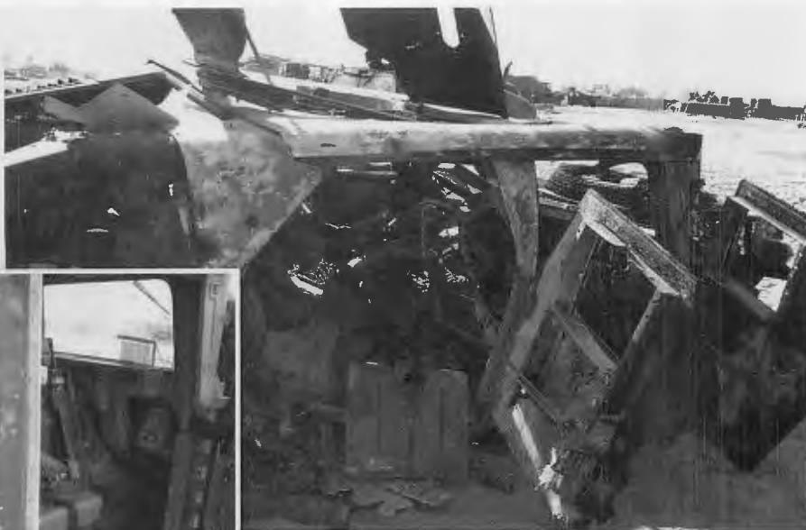
Barrett's front passenger seat before and after the blast from an IED. The armored doors withstood the explosion, although armored windows are gone.
