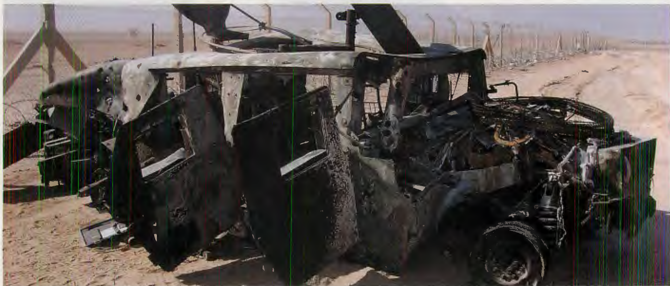
Barrett’s humvee after the IED detonated. Note the bent roof and sagging doors. Miraculously, all the Marines inside survived.
